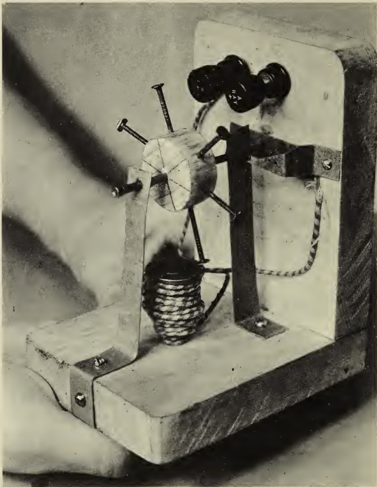
Fig. 28. The completed motor ready for action. The round black objects at the top are binding posts. The battery can be connected to two binding posts such as these or two small machine screws can be used. If the builder wishes, he can also make his battery connections direct. The binding posts or screws are not essential.
